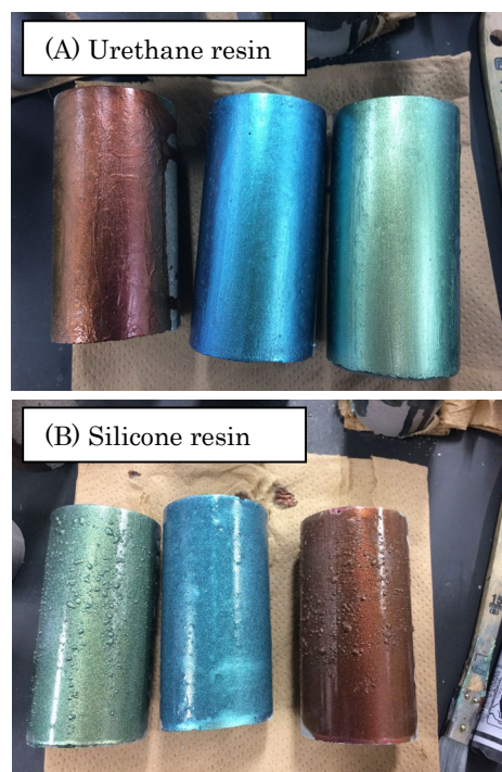
Figure 1. Photographs of SCPs on the concrete surfaces, (A) Urethane and (B) Silicon resins.
