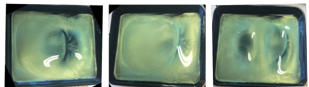
Figure 6. The variation of optical texture of SCP dispersed in Silicon oil as a function of the vibrational frequency.
