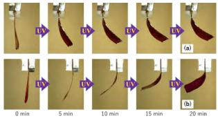
Figure 2 Variation of shape in PSPLG gel linked with 8 mol%-(a) PEHA and (b) DATD as a function of irradiation time of UV light.
