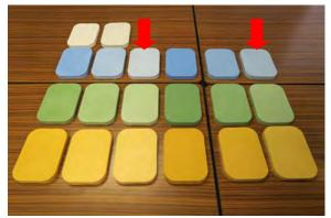
Photo4 Colors of specimens at the age of 6 months (Comparing the colors of the specimens with 1/4 of the manufacturer recommended pigment dosage, which are indicated by the red arrows, the specimens with W/B of 0.5 become lighter in color than the specimens with W/B of 0.2 over time)
