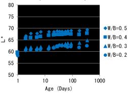
Fig. 2 Example of color changes over time (Blue specimen: L\* value)
