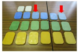
Photo3 Colors of specimens at the age of 1day (Comparing the colors of the specimens with 1/4 of the manufacturer recommended pigment dosage, which are indicated by the red arrows, the specimens with W/B of 0.5 are darker in color than the specimens with W/B of 0.2.)
