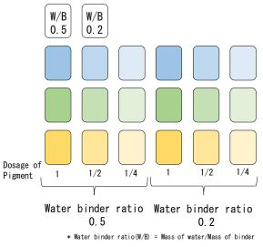
Fig.3 Parameter of experiment
