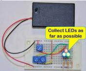
Fig.2. Lighting LEDs to confirm circuit correct
