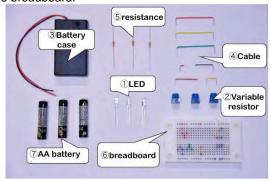
Fig. 1 Electric parts of this craftwork
