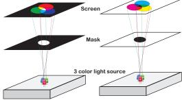
Fig.4. Basic arrangement of the color mixer
