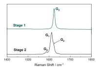
Fig.6 Raman spectra of stage 1 and 2 MoCl<sub>5</sub>-GICs.
