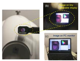
Fig. 1 (a) Photograph of TIAS using one eye of the wearable display, (b) tongue image on the wearable display (subject person side), and (c) tongue image indicated on the medical practitioner's computer.
