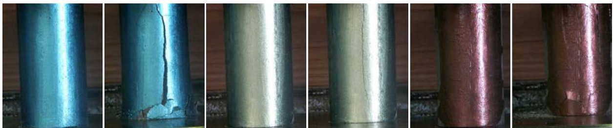
Figure 3. Comparison of colors in SCP-urethane paint before and after destruction of concrete.
