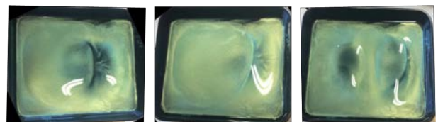
Figure 6. The variation of optical texture of SCP dispersed in Silicon oil as a function of the vibrational frequency.
