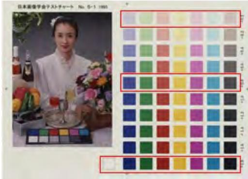
**Fig. 2 Test chart No. 5-1 of the Imaging Society of Japan (color patches surrounded by red frames were measured)**
