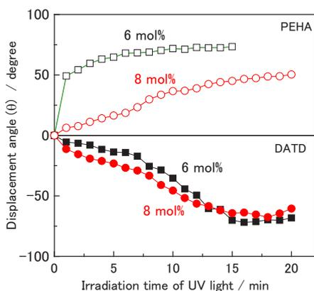
Figure 3 Variation of the displacement angle  $\theta$  of (a) PEHA and (b) DATD gel actuators as a function of 365 nm light exposure time.
