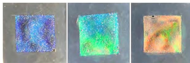
Figure 5 Photographs of Structural colors obtained from HPC solution.
