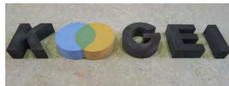
Photo2 University logo mark made from colored concrete (Colored mortar)
