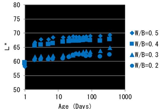
Fig. 2 Example of color changes over time (Blue specimen: L\* value)
