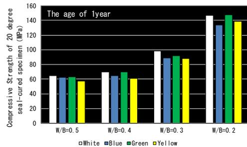
Fig. 1 Compressive test results of Colored concrete (Colored mortar)
