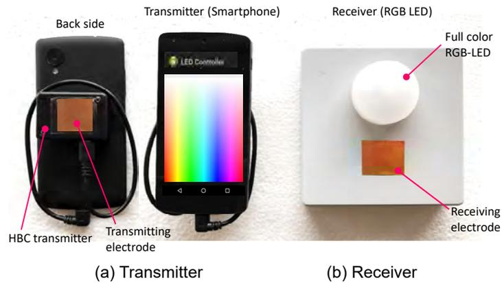
Fig. 2 A prototyped human body communication system
