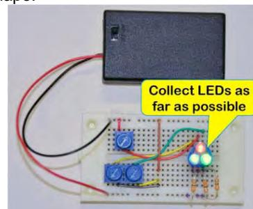
Fig.2. Lighting LEDs to confirm circuit correct
