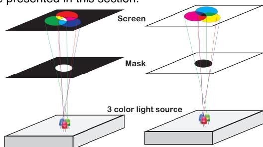
Fig.4. Basic arrangement of the color mixer
