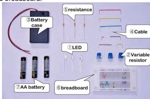
Fig. 1 Electric parts of this craftwork
