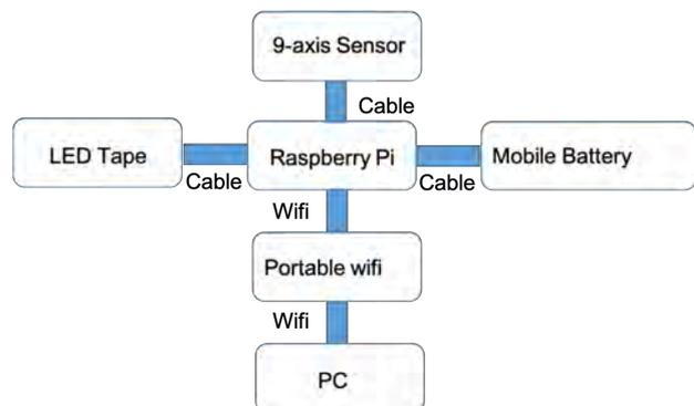
Fig.2 The system configuration.
