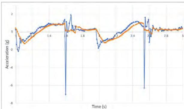
Fig 3. The graph of the original acceleration X-axis of the pole for 2 seconds (blue) and the moving average after 10 times (orange) in the beginner's Nordic walking.
