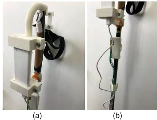
Fig.1 The appearance of the system. (a) The mobile battery is attached to the top of the Nordic walking poles. (b) Raspberry Pi Zero W, 9-axis sensor, and the LED tape are attached under the mobile battery.
