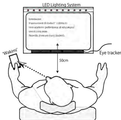
Fig. 1 The smart LED lighting system
