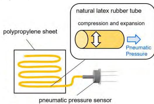
Fig. 2 Principle of the pneumatic pressure sensor.
