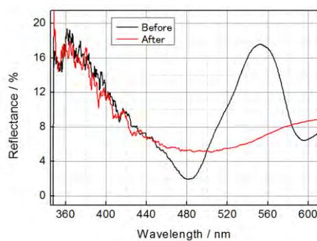
**Fig. 3** Specular reflectance spectra of the pigment film (thickness : 80 nm) before and after the photo-illumination.
