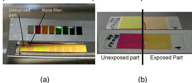
**Fig. 1** Photograph of the safflower red pigment film (thickness : 0.4  $\mu\text{m}$ ) on the quartz crystal plate demonstrating the effect of photo-illumination through multi-color filter for 30 minutes. (a) **Fig. 2** Photograph of the pigment film (thickness : 80 nm) after the long (139 min.) photo-illumination.(b)
