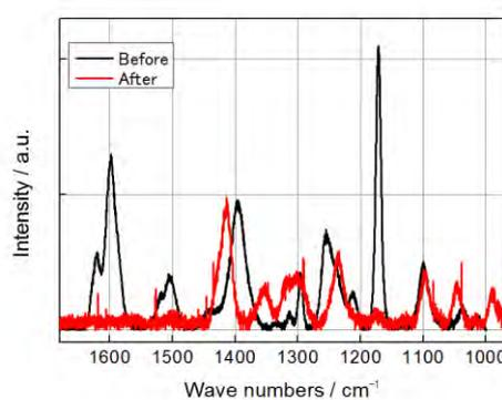
**Fig. 4** Raman spectra of the pigment film (thickness : 80 nm) before and after the photo-illumination.
