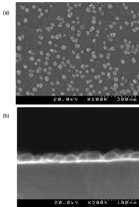
**Fig. 1 FE-SEM surface (a) and cross-sectional (b) images of the ITO electrode after electrodeposition of Au with pulse voltage application of -12 V.**
