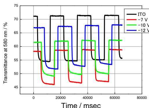
**Fig. 4** Time courses of transmittance at 580 nm for PEDOT/Au-ITO devices induced by polarity inversion of applied voltage (2.5 V).
