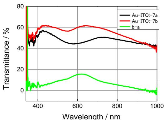
**Fig. 2** Changes in transmittance spectrum of Au-ITO device induced by DC voltage switching between -2.5 V and +2.5 V.
