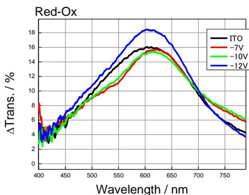
**Fig. 3** Difference spectra for PEDOT/Au-ITO devices induced by polarity inversion of applied voltage (2.5 V).
